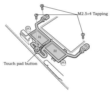
Figure 4-18 Removing the touch pad button
